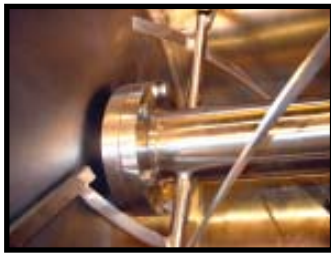
Agitator with Flanged Journal Construction
