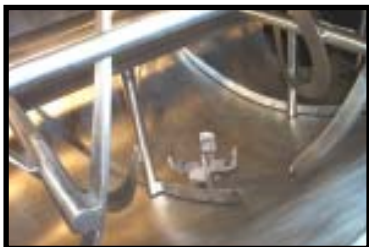
High Velocity Intensifiers to break up lumps
