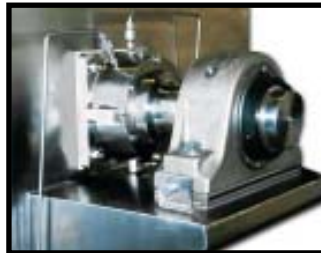
Packing Gland Seal with Air Purge
