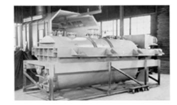
Thermal treatment is provided through a thermal fluid jacket on the mixing vessel. Material is heated or cooled by direct contact with the surface area on the tank walls as the paddles and/or ribbons continuously agitate the material. Based on standard models, our engineers can design a heating or cooling mixer to your specific processing needs.
